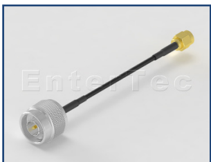
Con1: N(M) S/T Plug Cable: RG-174 Con2: SMA(M) S/T Plug
