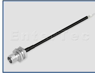
Con1: TNC(F) S/T Bulkhead Jack With O-Ring Cable: RD-174 Con2: Strip&Tin
