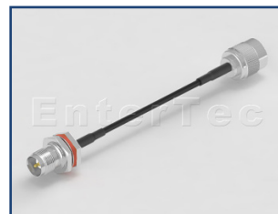
Con1: TNC(F) S/T R/P Bulkhead Jack With O-Ring Cable: RG-174 Con2: TNC(M) S/T R/P Plug
