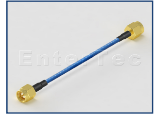
Con1: SMA(M) S/T Plug Cable: Semi-Flexible RG-405 Con2: SMA(M) S/T Plug
