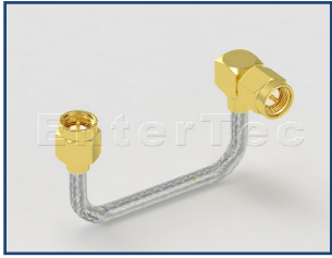
Con1: SMA(M) S/T Plug Cable: .141 Semi-Flexible RG-402 Con2: SMA(M) R/A Plug
