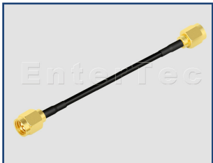
Con1: SMA(M) S/T Plug Cable: LMR-195 Con2: SMA(M) S/T Plug
