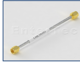
Con1: SMA(M) S/T Plug Cable: .141 Semi-Flexible RG-402 Con2: SMA(M) S/T Plug
