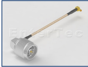
Con1: N(M) R/A Plug Cable: RG-316 Con2: MMCX(M) R/A Plug
