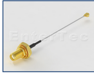
Con1: SMA(F) S/T Bulkhead Jack With O-Ring Cable: 0.81mm Con2: IPEX(2.5H)
